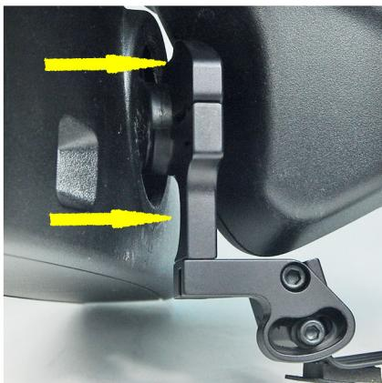
**4** While sitting in the passenger seat, place the mount over the mirror stem. Tighten the CLAMP SCREW until the mount starts to clamp onto the mirror stem. Position the mount as far forward as it will go and parallel to the bottom of the mirror before fully tightening.
